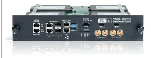
The innovative CMS-2200 Cinema Media Server for the digital cinema industry supports JPEG-2000 decoding of 4K and high frame rate 2K images with advanced solid state storage. Two USB 3.0 ports enable accelerated ingest of content and live streaming. The system is HDMI 2D & 3D compliant.
